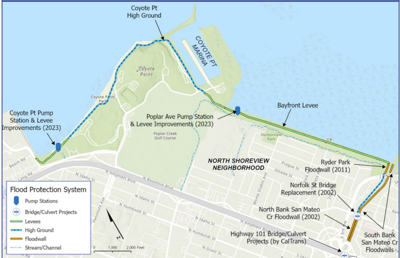
Figure S-11 North Shoreview Flood Protection Improvements
