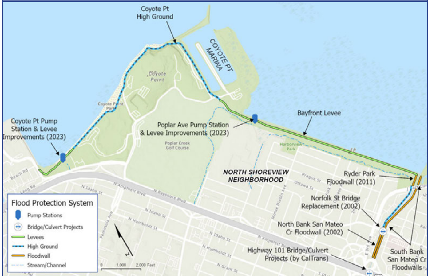
Figure S-11 North Shoreview Flood Protection Improvements
