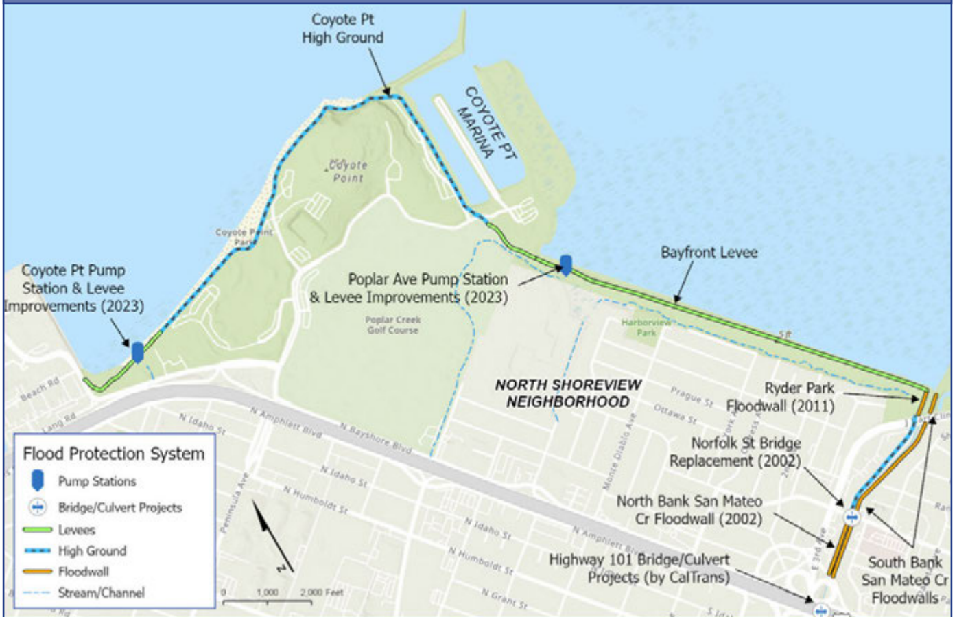
Figure S-11 North Shoreview Flood Protection Improvements
