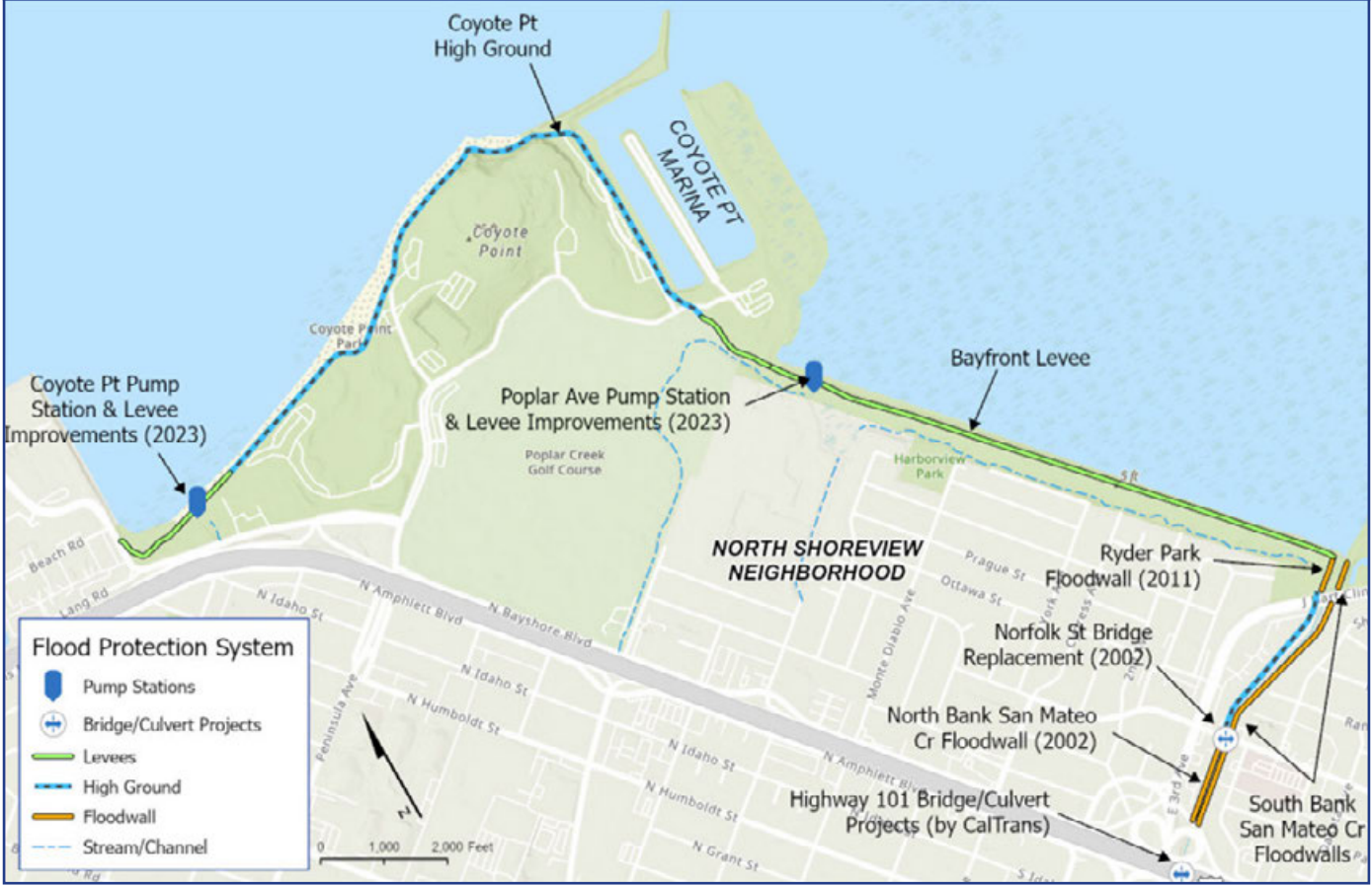
Figure S-11 North Shoreview Flood Protection Improvements
